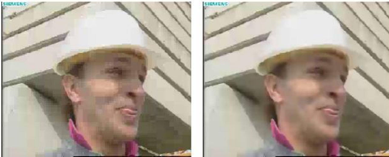
Figure 4 Performance of the deblocking filter for highly compressed pictures. Left: without the deblocking filter. Right: with the deblocking filter.
